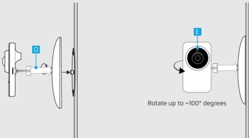
**D** Press the foot of the camera on the white plastic mounting plate (The metal ring does not have to be placed back). Screw the stand of the camera back on the foot and tighten it.
