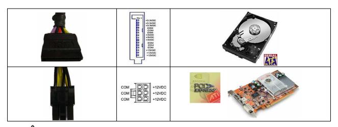
Refer to the manual of motherboard, peripheral, drive or interface card for correct power connection!
